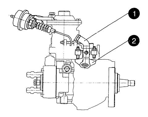
Position (arrow) LFG stop lever (1) against screw for low idle. Adjust dimension A (curved end of basic lever – pump flange) at LFG basic lever (2). Tighten hexagon nut to 3...5 Nm and fillister—head bolt to 5...7 Nm.
